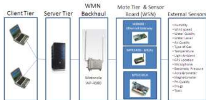
Fig. 5: End-to-end application block diagram
